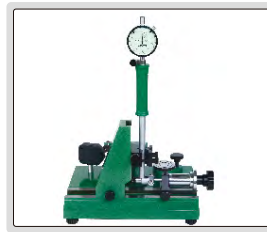
inspect accuracy of dial bore gages (range 6-450mm)
