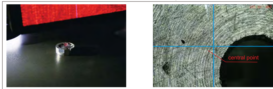
laser indicator locates the central point
