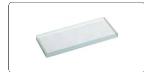
50mm reading scale (check magnification accuracy)
