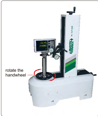
rotate the handwheel to rotate tools
