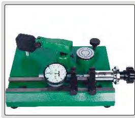
inspect accuracy of dial indicators (range 0-25mm)
